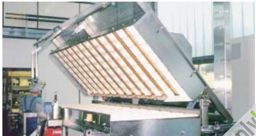
*Heat treatment of glass fibre material prior to further processing*
