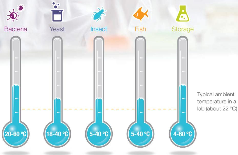
Thermo Scientific refrigerated incubators provide optimal temperature environments for applications that require stable temperatures above or below ambient, including incubation of bacteria, yeast, insects or fish, and temperature storage. They are also optimal for standard 30 to 37 °C incubation applications in warm environments.
