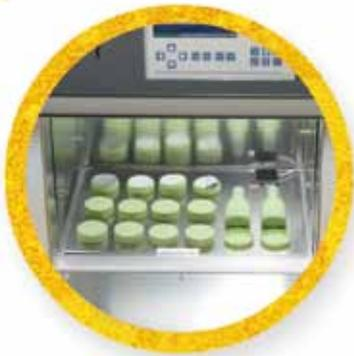
Flatbed testing technology allows for the testing of almost any shape and size. The optional accessories for lowering the sample temperature are helpful tools for photostability testing of thermal sensitive products, pharmaceuticals or cosmetics.
