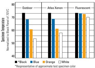
Note: Black Panel temperature in the fluorescent device is achieved only by heating the chamber air (no IR). Thus, all specimens are heated equally, without regard to color. Because xenon light is a full spectrum light source like natural light, sample temperatures vary by color, as in natural sunlight.
