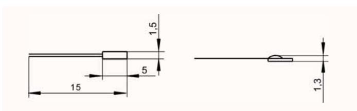
Unprotected sensor element for constructing your own sensors
