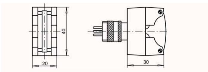
For surface measurement on convex / concave surfaces
