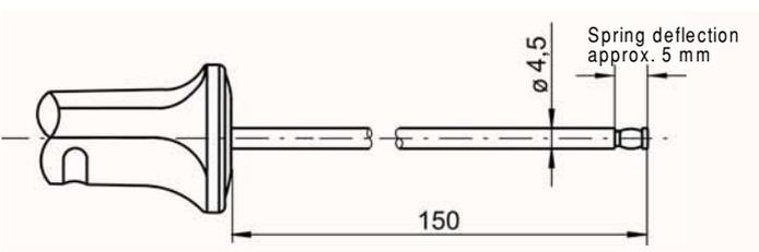
For surface measurement on level, metallic surfaces
