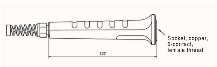
Built-in socket For circular connectors with screw connection
