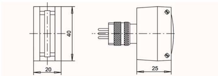
For surface measurement on level surfaces
