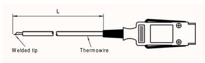
For surface measurement and immersion measurement
