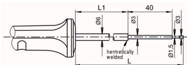
For surface measurement and immersion measurement
