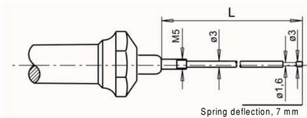
For surface measurement and immersion measurement
