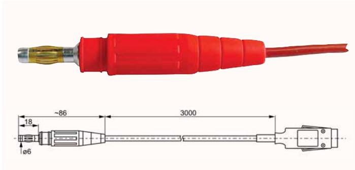
Measuring element PT100, 4-conductor class B, integrated in the socket of a 6 mm laboratory connector made of brass (nickel-plated).
