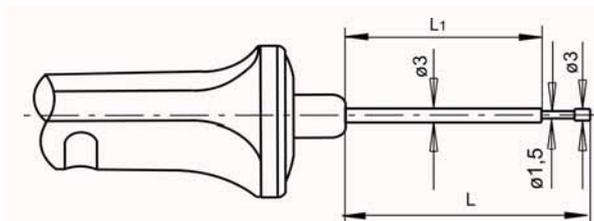
For surface measurement and immersion measurement
