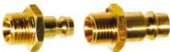
Quick-release coupling nominal width 7.2 external thread G1/4"
